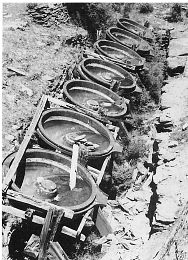
Fig. 11: A row of seven berdans at the Invincible mine site, Rees Valley, central Otago, South Island, New Zealand (N. Ritchie).
